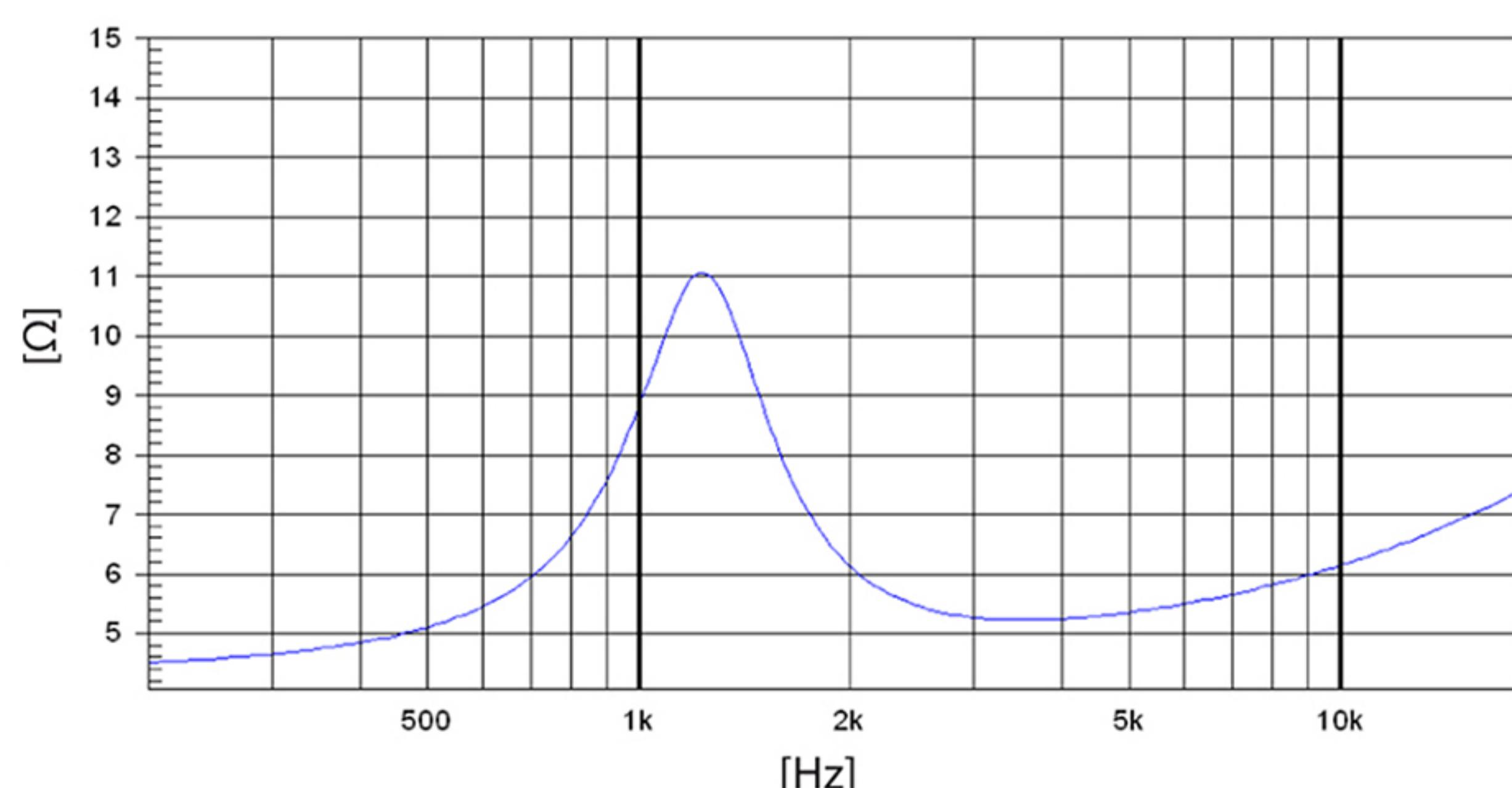
Note: Electrical impedance measured coupled to: M 212 horn
