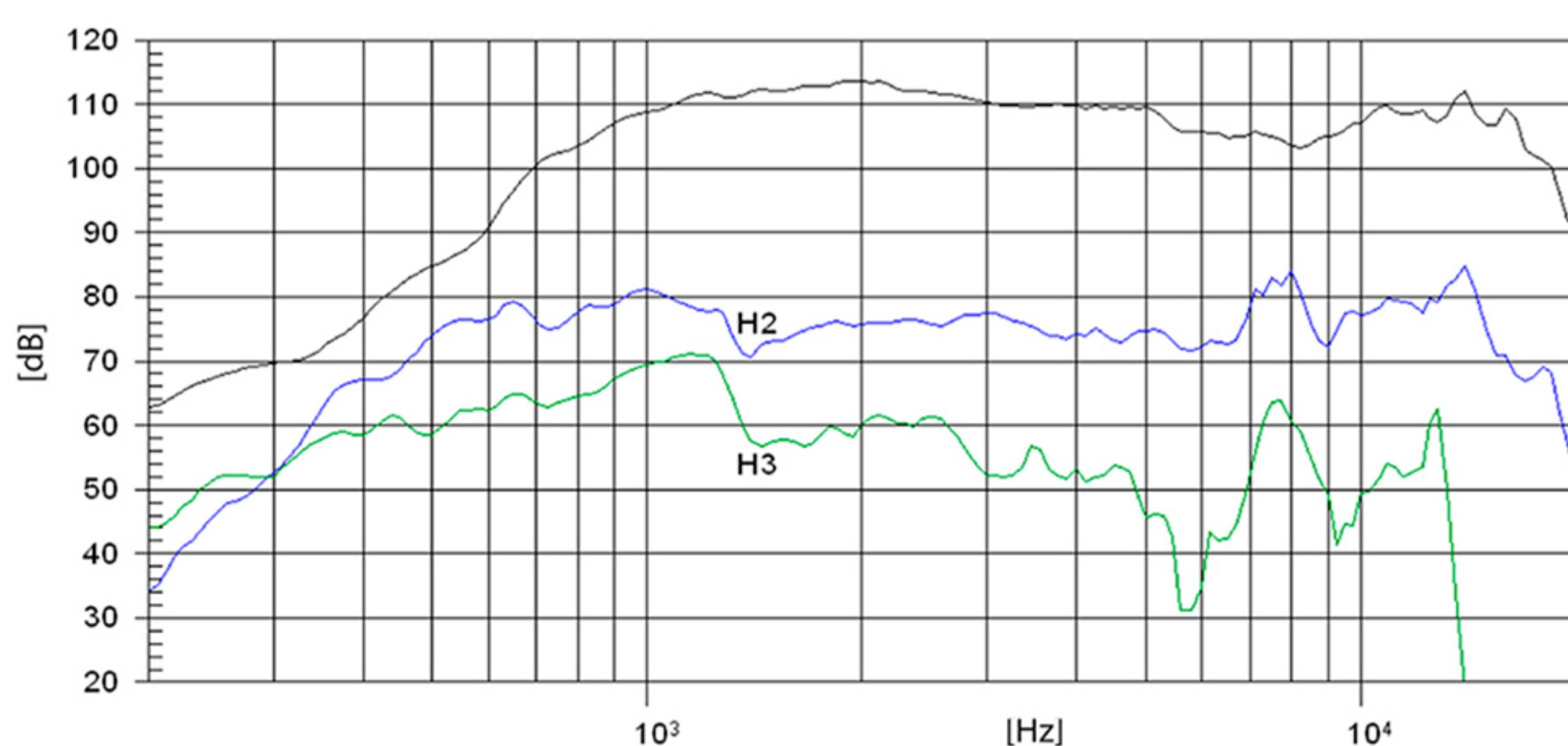
Note: On axis frequency response measured coupled to: M 212 horn in anechoic chamber, 2,83 v @ 1m
